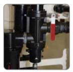
**Remote Control Valves** Used with a deadman's handle, the  $1\frac{1}{2}$ " (38mm) remote control valve minimises air flow loss and shuts the blast system down quickly and safely.
