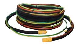
Elcometer Blast Hose Assemblies contain twinline remote control hose, DMHII deadman's handle, nozzle holder and quick coupling. Blast hose assemblies are available in either 174psi (12bar) or 217psi (15bar) working pressure.
