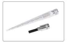
The Elcometer 103 Blast Nozzle Gauge measures the orifice size of an abrasive blasting nozzle. This gauge is used to determine the nozzle orifice wear which leads to low nozzle pressure and decreased efficiency in its performance. Nozzle orifice wear results in decreased productivity and increased abrasive media consumption.
