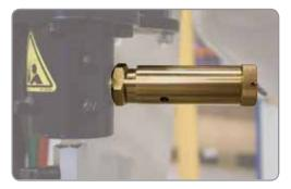
Pressure relief valves must be incorporated into the blast machine system to meet global safety standards. Elcometer's certified pressure relief valves can be easily fitted to the air manifold which is fitted to the RCV4000+ remote control valve. Pressure relief valves are designed to discharge the compressed air in the blast machine upon reaching the crack pressure.
