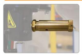
Pressure relief valves must be incorporated into the blast machine system to meet global safety standards. Elcometer's certified pressure relief valves can be easily fitted to the air manifold which is fitted to the RCV4000+ remote control valve. Pressure relief valves are designed to discharge the compressed air in the blast machine upon reaching the crack pressure.
