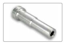
Designed to create a wide blast pattern and increased velocity, the Tungsten Carbide Venturi Blast Nozzle with Aluminium Jacket is ideal for blasting large surfaces. Supplied with a rubber gasket, this general purpose blast nozzle features a tungsten carbide insert and aluminium jacket providing durability and toughness.
