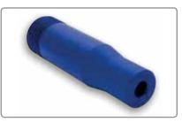
The Silicon Carbide Venturi Nozzle features an acetal jacket offering high impact protection. Designed to have a prolonged lifespan, this nozzle is ideal for use with harder abrasives such as chilled iron and aluminium oxide. Supplied with a rubber gasket, the nozzles have a silicon carbide liner which offers impact resistance and durability whilst remaining lightweight.
