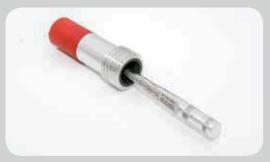
A small increase in the nozzle size will result in a very large increase in air and abrasive consumption and adversely affect blasting efficiency. To ensure your nozzle provides continuous high production, as a general rule, replace your nozzle when the orifice wears by 1 nozzle size, when a #2 nozzle becomes the size of a #3 nozzle, for example.
